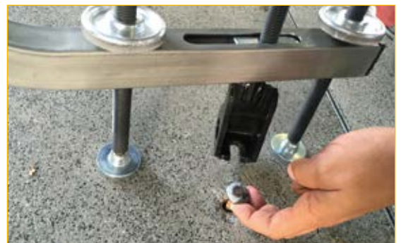
Central tie rod with rotating and sliding hook. In central picture visible female coupling.
